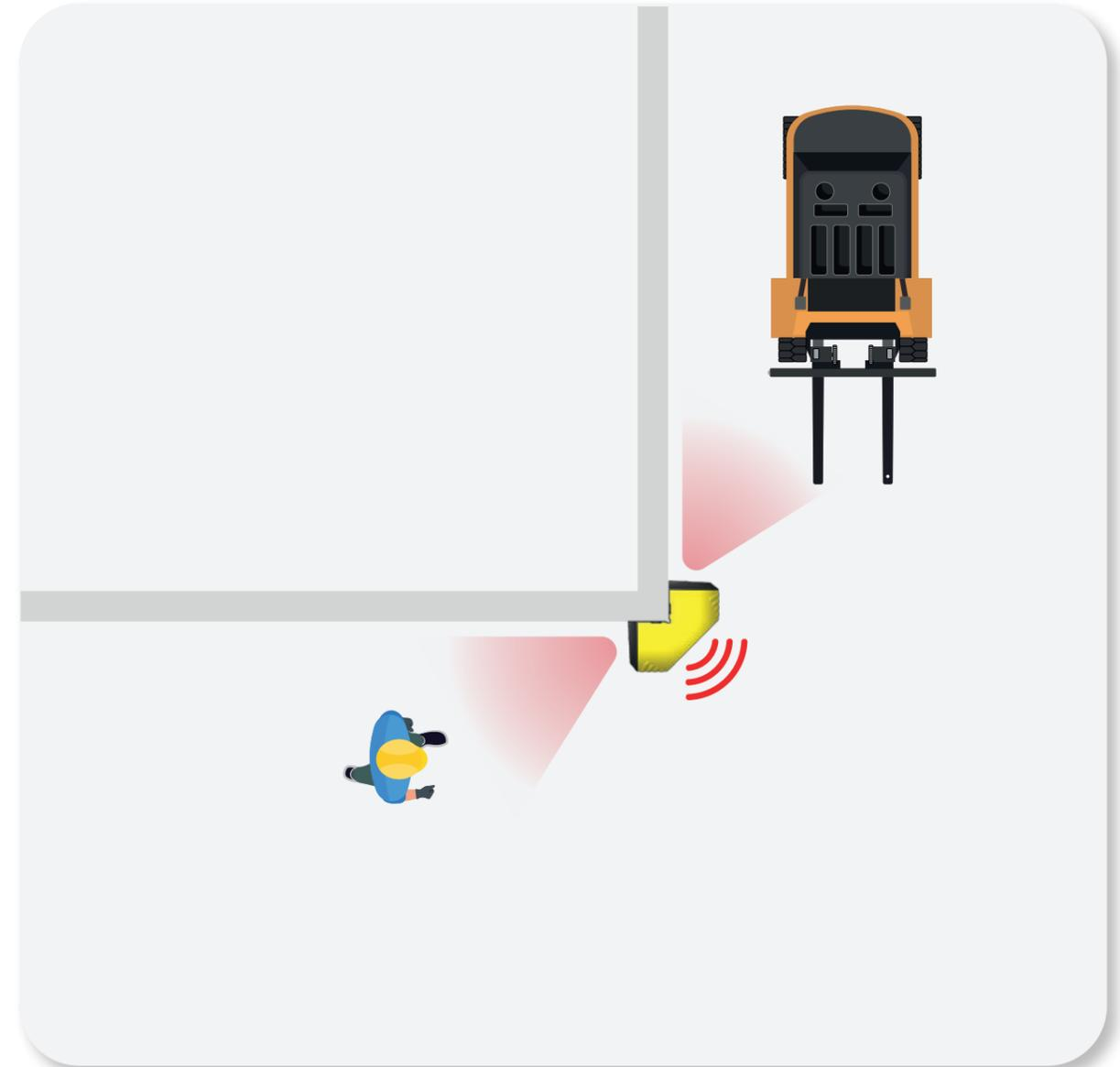
Our SHUTTLE can warn you of Possible collisions around corners. It can detect incoming traffic from both ends and, if a collision is possible, will warn you with audio and visual cues. It can spot all types of moving object, from the largest to the smallest.
