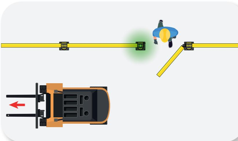
Safe Way allows passage when the vehicle no longer poses a danger.
